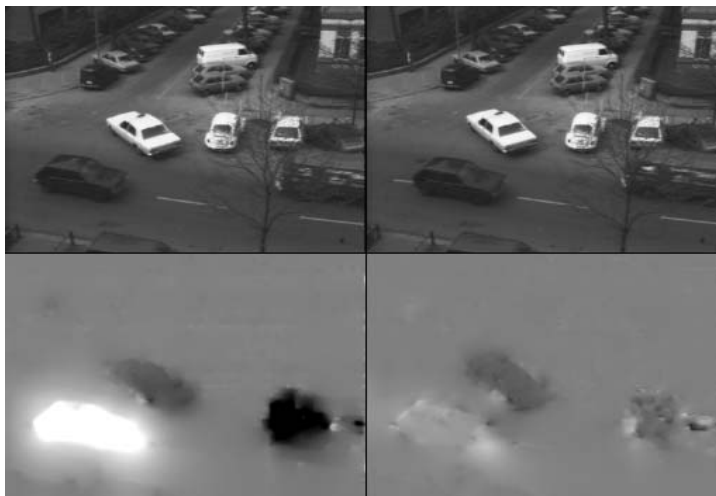
Figure 1: Numerical Experience. Up: we present two frames of a movie sequence. Down: We present the computed optical flow u_{i,j} (left) and v_{i,j} (right) using our method for the quadratic term. When the grey level of the images go to the white indicates a displacement of the object toward the right in the case of u_{i,j} or toward the down in the case of v_{i,j} . In the same way, when the grey level of the images go to the black, it indicates a displacement of the object toward the left in the case of u_{i,j} or toward the up in the case of v_{i,j}
