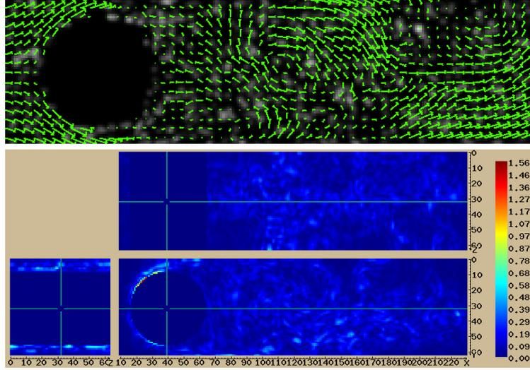
Fig. 4. Top, real flow. Bottom, final error distribution (combined scheme).
